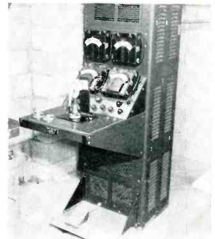
Production type core tester (left) has automatic testing features. Yield at first operational test point increased from 70 to 90 percent on introduction of this method. Developmental model of core tester is shown at right
