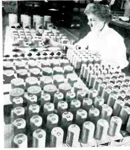
Operator applies finishing touches to a group of nickel-iron alloy cores (left) while another operator inspects finished group of magnetic amplifier reactors (right)
