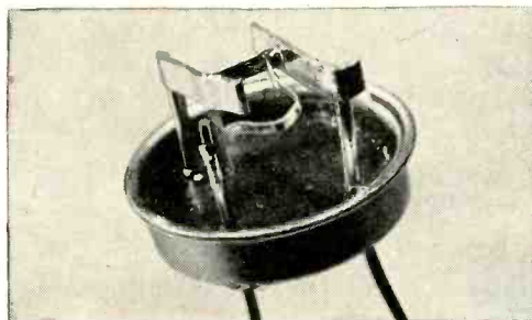
View of uncapped G-E silicon NPN diffused-meltback transistor, showing mounted silicon bar with aluminum base lead connected. Bar ends attached using a gold-alloy mounting technique. No solders or fluxes are used.
