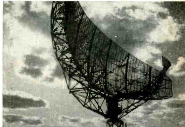
WAYLAND LABORATORY engineers developed this 40-foot L-band antenna to extend the range of radar.
