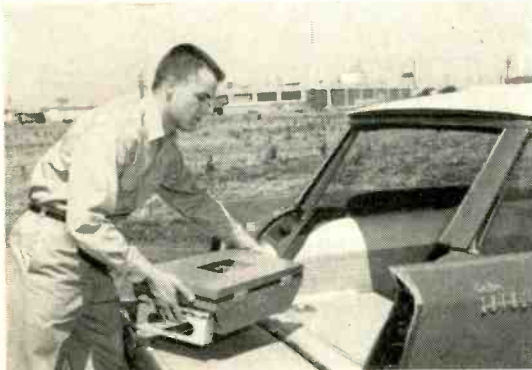
Ampex 800 tape transport, showing small size and ease of handling. This is the largest of the recorder components.
