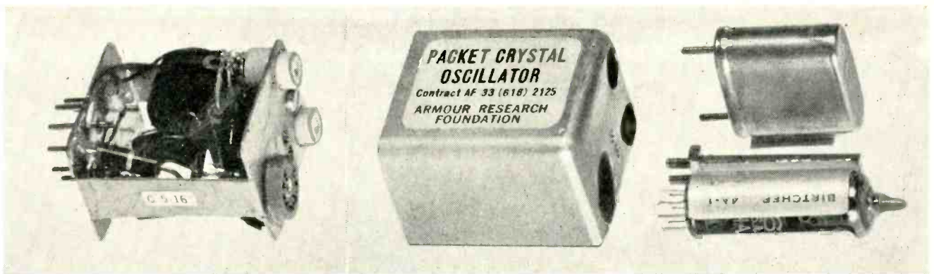
Plug-in unit fits into the standard nine-pin noval socket. Base is hermetic-seal structure \frac{7}{8} \times 1 \frac{1}{16} in., with overall height 2\frac{5}{8} in.
