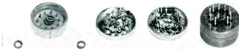
Packaging of Ferractor headers and other circuit components. Header at left shows how two cores, representing independent amplifiers, fit into hermetically sealed unit
