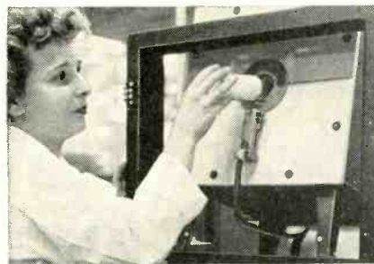
Diffusion furnace. Operator places quartz vials, with large quantity of silicon bars, in furnace. Diffusion occurs through high-temperature heating cycle lasting several hours.
