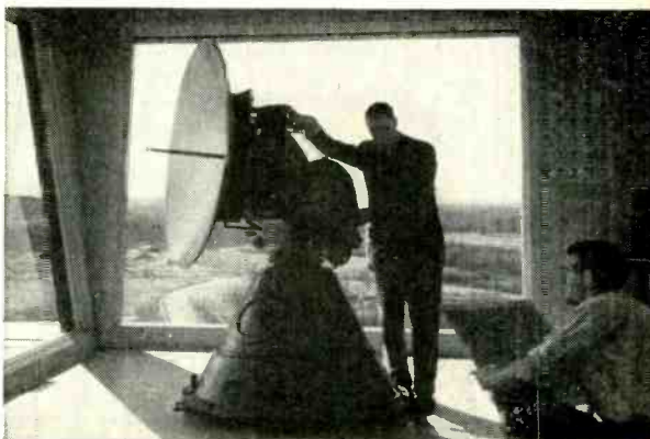
MISSILE SYSTEMS DIVISION facilities include observation tower with radar tracking equipment.
