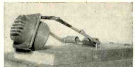
Large circular AN connector is held firmly even when square mounting flange is not resting on base of trap
