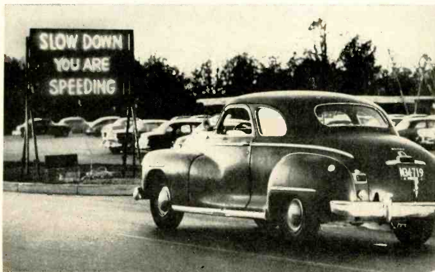
NEON sign, hooked to radar timer, lights up, driver slows down when . . .
