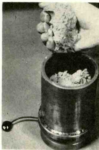
STEP 4. Can in position over mold to serve as funnel for applying filler
