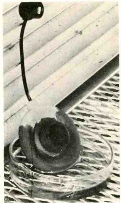
STEP 7. Coil resting in small dish absorbs resin quickly
